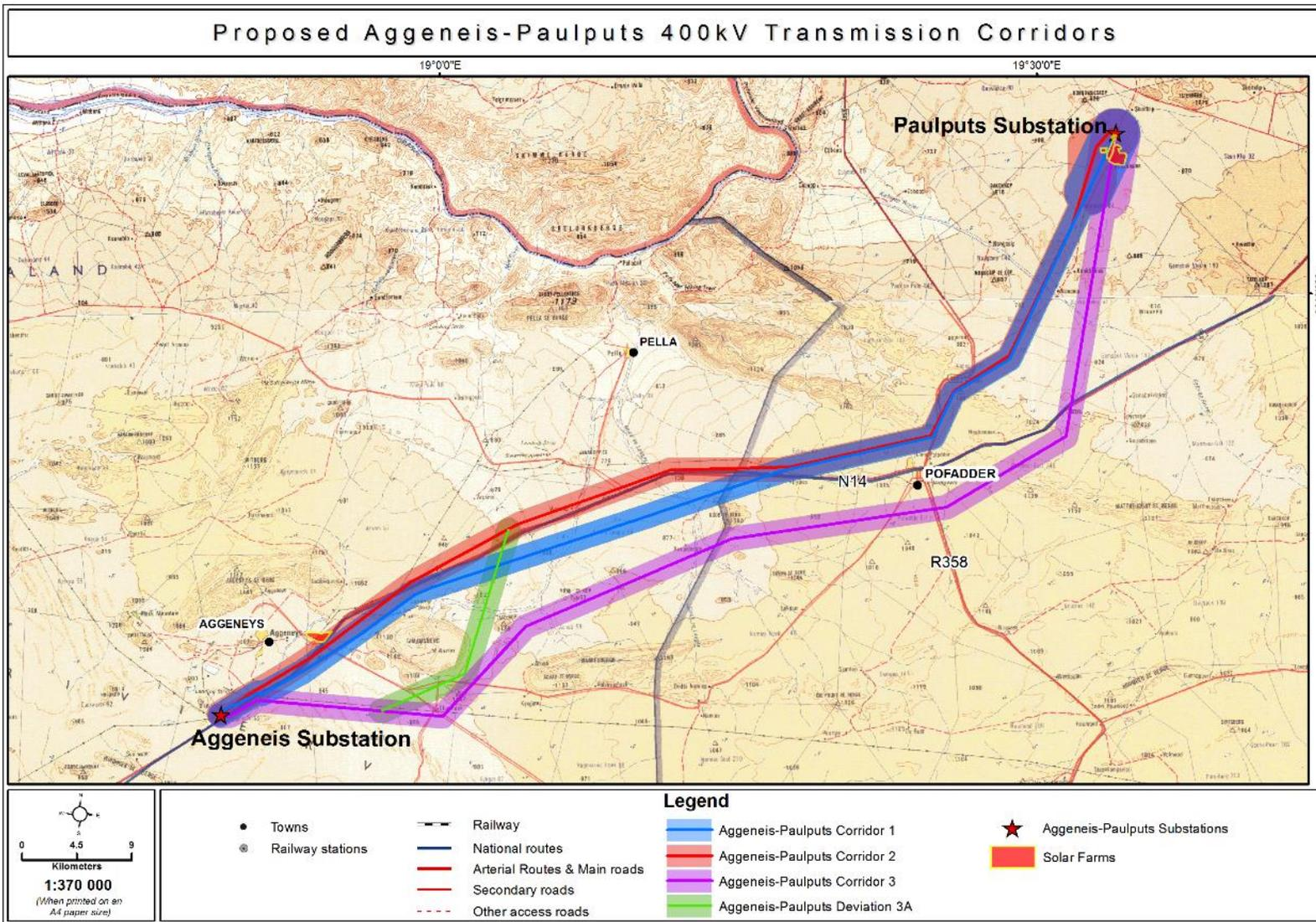
Figure 1: Locality map for the alternative corridors, and deviation 3A
